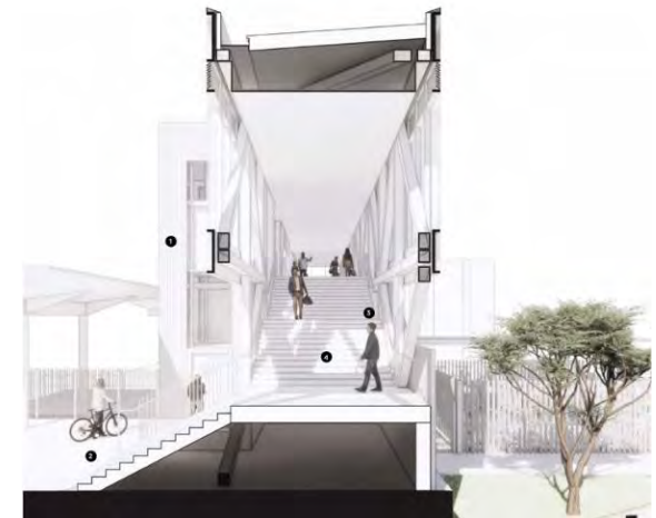
Figure 40: Depiction of overpass entry with lift tower pictured on the left-side of the entrance
